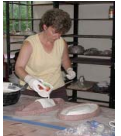
Mills pours plaster over a one-part mold during "The Cast Vessel" workshop at Peter's Valley Craft Center in Layton, NJ.
